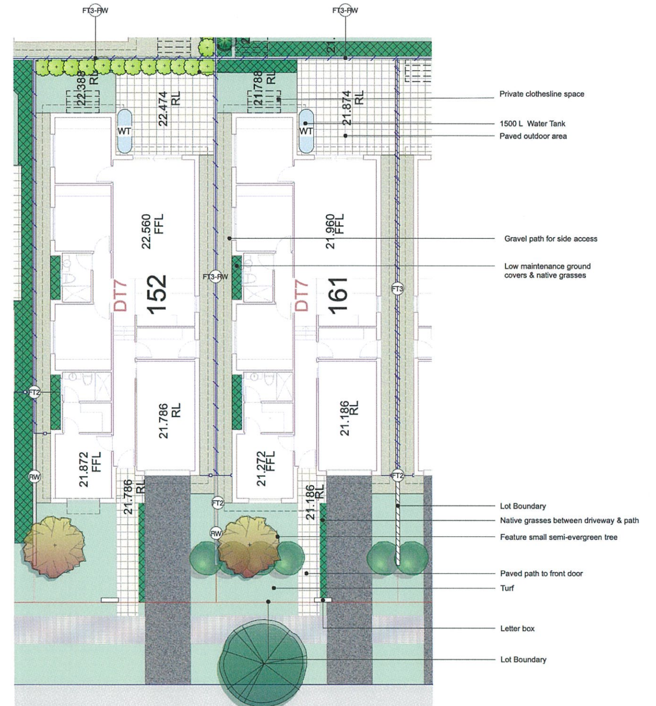
2 TYPICAL 4 BED SINGLE STOREY - SINGLE GARAGE Scale 1:100
