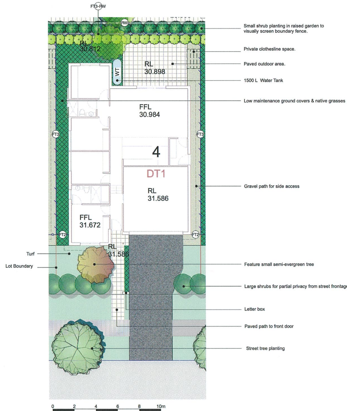
1 TYPICAL 4 BED SINGLE STOREY - DOUBLE GARAGE Scale 1:100
